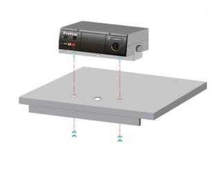
There are three holes on the front cabin sheet. Thermocouples (sensors) of the control panel (thermostat, safety thermostat, thermometer) must be passed through the middle hole. Control panel must be stabilized to the holes on right and left.
