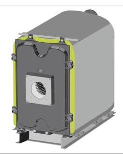
Isolation must be cut around assembling ears connection points.
